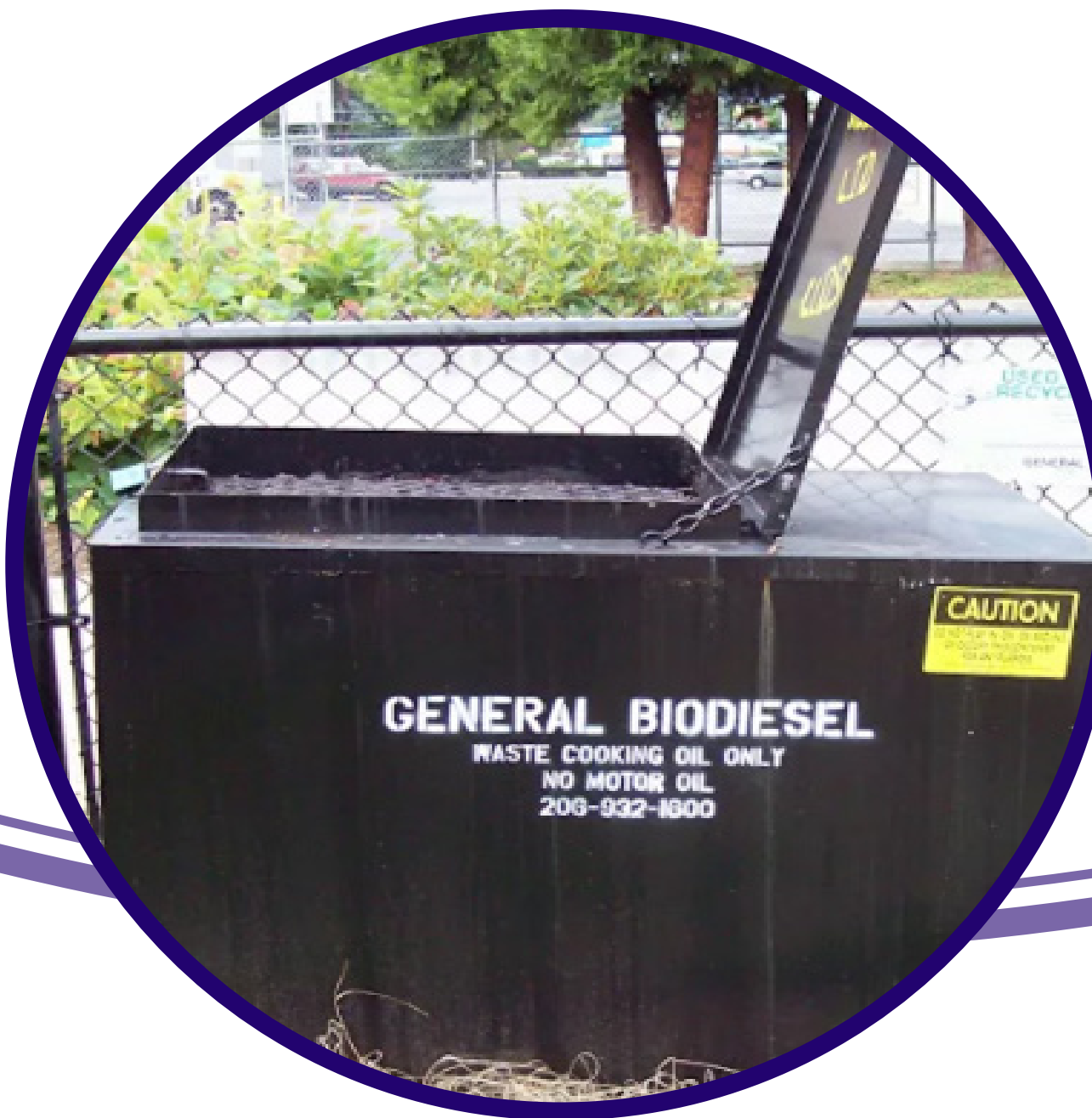
An example of a FOG collection bin. This bin is already in use in Auburn, located at the south end of Les Gove Park, north of SE 12th Street. Credit: City of Auburn
