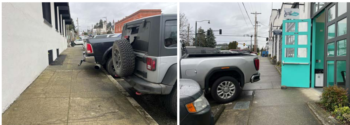
Figure 19. Angled and back-in curbside parking allows vehicles with large overhangs to block pedestrian mobility, greatly reducing sidewalk capacity and equal access.
