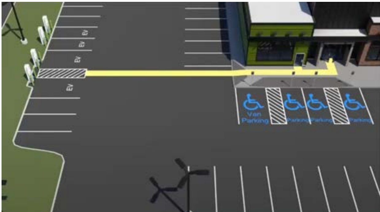
Figure 4.3. A direct and accessible route from the charging station to nearby amenities.
